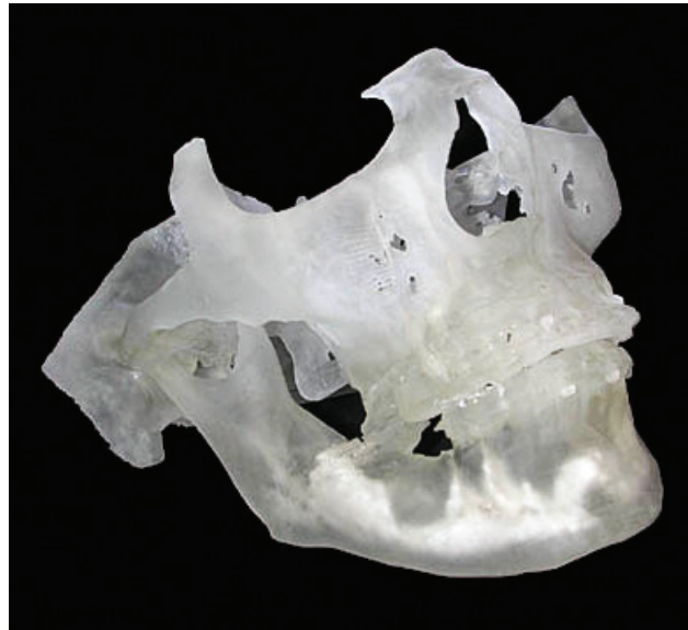
Figure C2: Physical prototype made using stereo lithography
